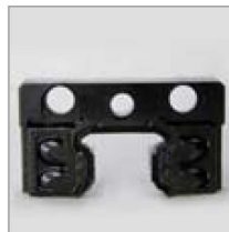
End seal in good condition
